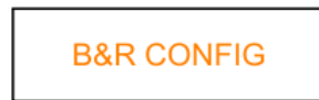
Figure 6.26: The configuration block. It must be always present (only once) in the Simulink model.
