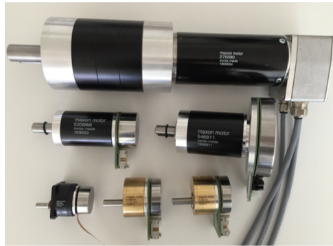
Figure 2.7: The six joints. One joint is composed by the motor, the gear and the encoder. The sixth joint hasn't got the encoder.
