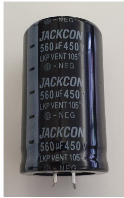
Figure 3.3.42: Jackcon LHK Series 560\mu F , 450 V , 105^\circ C aluminum electrolytic capacitor [29].
