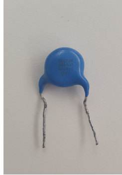
Figure 3.3.55: 2.2 nF, 2 kV single layer ceramic capacitor for turn-off snubber.
