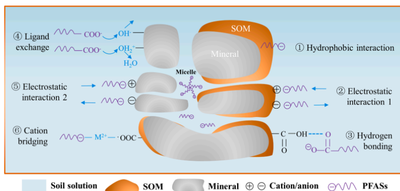
Fig. 1. Possible sorption behaviors of PFAS in the soil environments (an example of anionic PFAAs).
