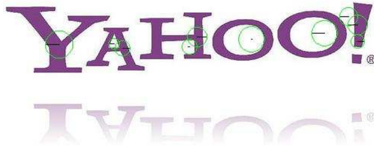
Figure 6.5. This is a simple image with some features points plotted. To understand the Proportional Technique you have to image to compute the distance between each of these points. They will be stored in a matrix of distance.
