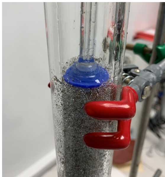
Figure 10. Packing of the column with a mixture of wet Amberlyst-15 and 1 mm glass spheres.
