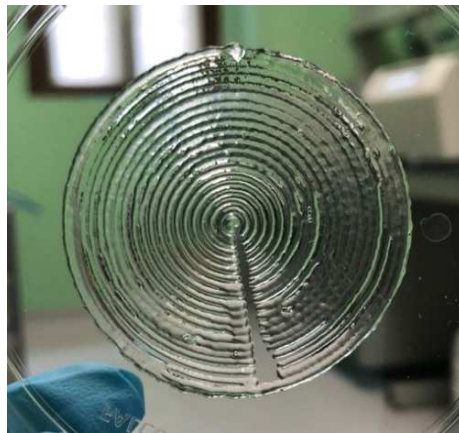
Figure 3.8 GelMA hydrogel sample with concentric geometry infill: the hydrogel distribution is discontinuous.
