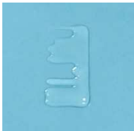
Figure 3.4 Right side of 8 channels ladder structure printed with 5% GelMA hydrogel.
