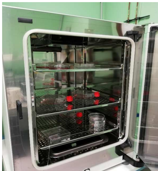
Figure 2.13 Incubator at 37 °C, with a 21% O 2 and 5% CO 2 internal environment, to cultivate cells.
