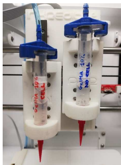
Figure 2.17 Extruder syringes loaded on the 3D bioprinter: on the left the one containing the cell-laden hydrogel and on the right the one with the hydrogel without cells; both are GelMA 10% hydrogel.
