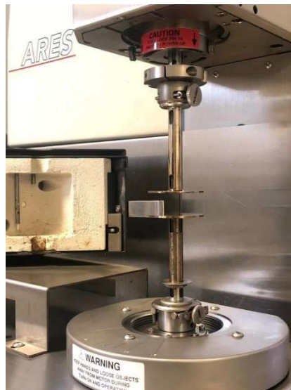
Figure 2.8 Rotational rheometer ARES-RFS used for mechanical test.
