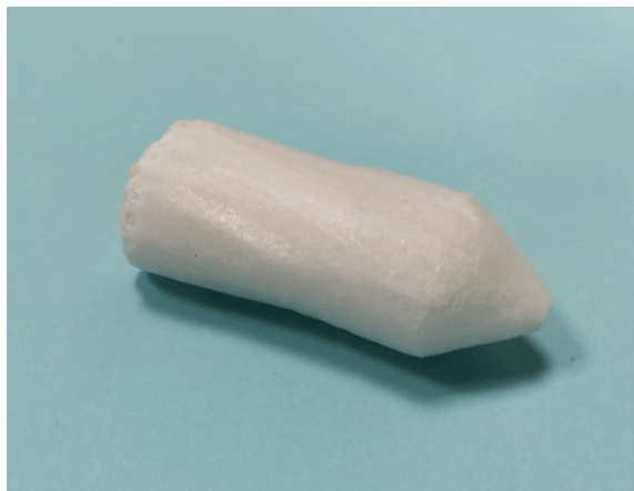
Figure 3.1 Gelatin methacrylate polymer synthesized with the Van Den Bulcke et al. (2000) method that provides dialysis and freeze-drying.
