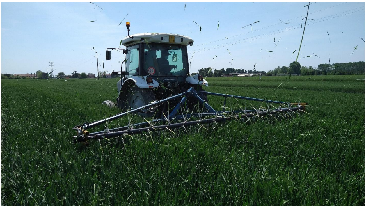
Figure 2: the first prototype while doing simulations of hail damage in winter wheat.
