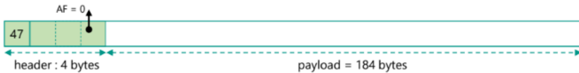
Figure 1.2: TS packet without adaption field.[Fis03]
