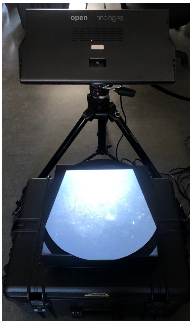
Fig. 17: scanner a luce strutturata Cronos Dual by Open Technologies
