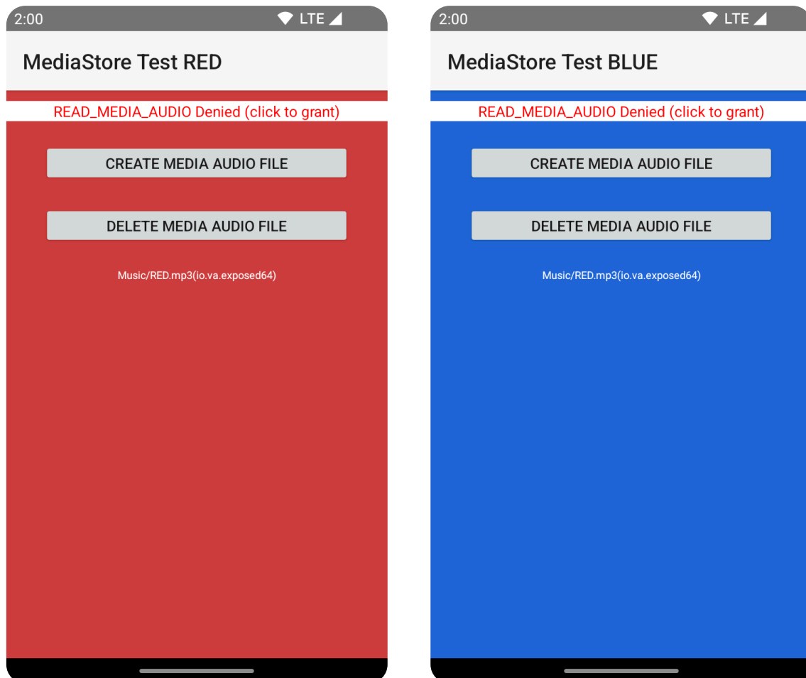
Figure 7 — Red creates a media audio file named RED.mp3. Blue is capable of querying also files created by Red, even if the permission Manifest.permission.READ_MEDIA_AUDIO is denied.
