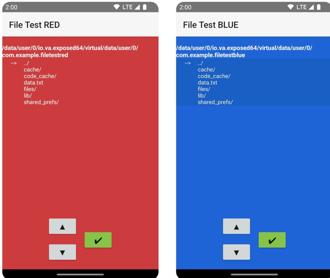
Figure 4 — com.example.filetestred and com.example.filetestblue , on the file manager. Each of the two apps points to their respective internal storage, on the redirected path.
