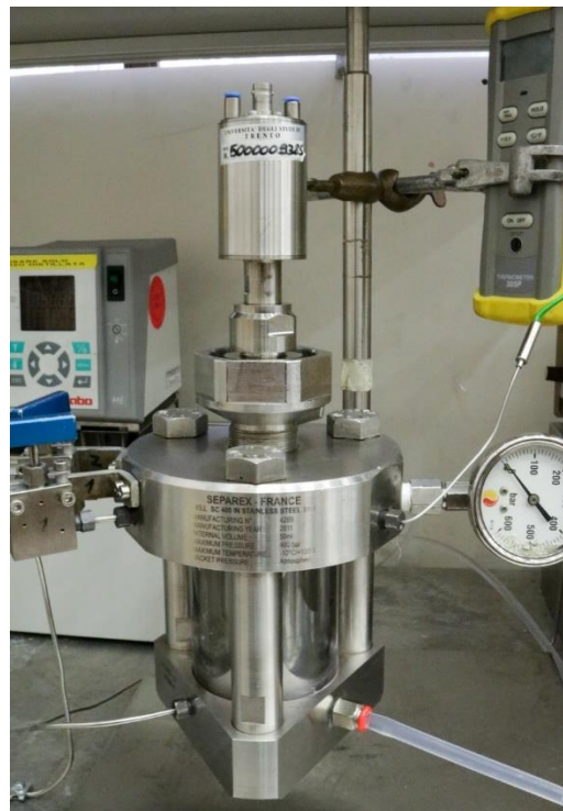
Figure 2.8 Modification of the HPCD reactor when the sonotrode is inserted.
