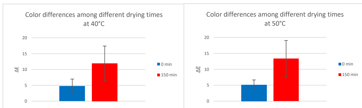
Figure 3.8. Color differences in terms of \Delta E among different drying times and temperatures (40°C and 50°C). Each point represents at least three independent measurements with the standard deviation of the mean.
