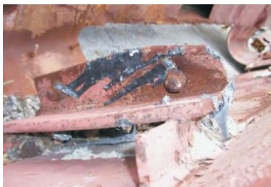
Figura 3.42. Condizione della vernice di primer sulla colonna 143 del pannello N-8 del WTC 1 (S.W. Banovic, T. Foecke (2006), Assessment of Structural Steel from the World Trade Center Towers, Part IV: Experimental Techniques to Assess Possible Exposure to High-Temperature Excursions).
