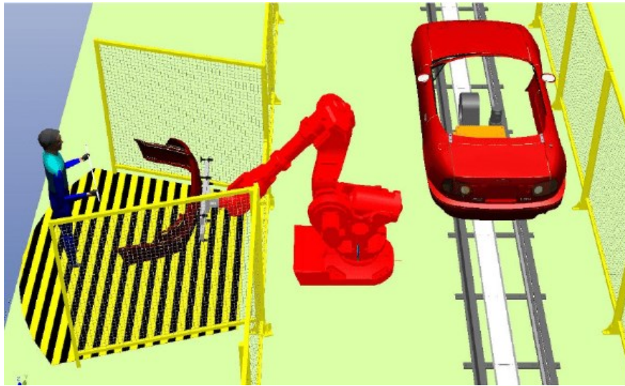
Figure 8: Safe standstill of an industrial robot for possible interaction with an Operator (Behnisch & Matthias, 2008)
