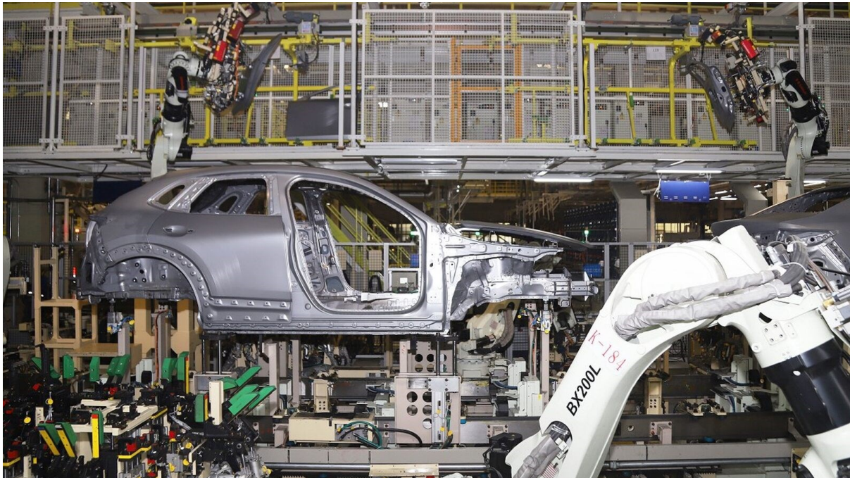
Figure 21: Automated solution for door/hood/lid assembly from Mazda Company (IFR, 2021)
