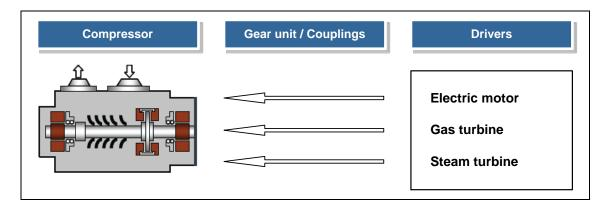
Figure 4.1: Drivetrain options for compressors
