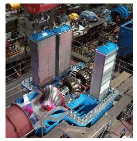
Figure 4.5: Radial isothermal compressor RIKT
