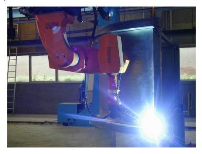
Figure 2.3: welding robot
