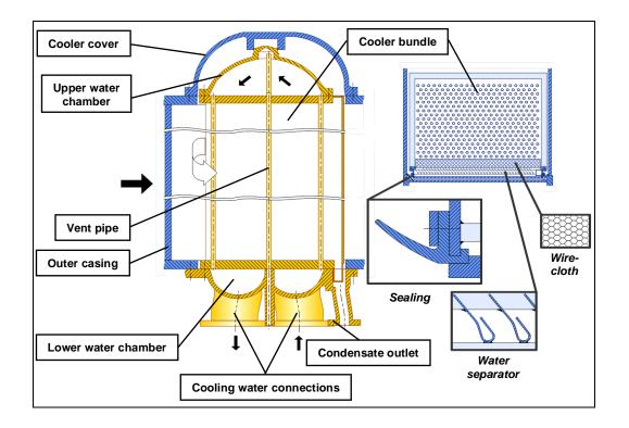
Figure 4.29: Intercooler - 2 water path
