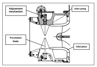
Figure 4.20: Inlet casing and inlet piece
