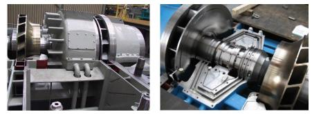
Figure 4.28: Bearing housing
