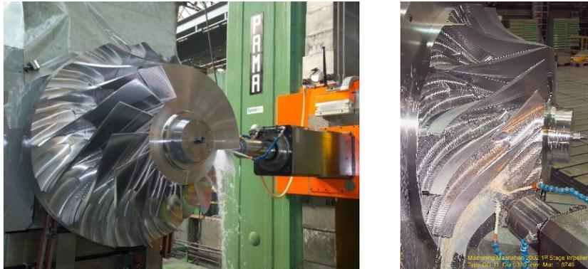
Figure 4.11: Milling impeller 1<sup>st</sup> stage
