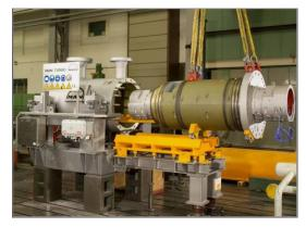
Figure 4.7: Centrifugal compressor with barrel design
