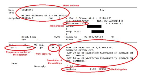
Figure 4.30: example of a work cycle
