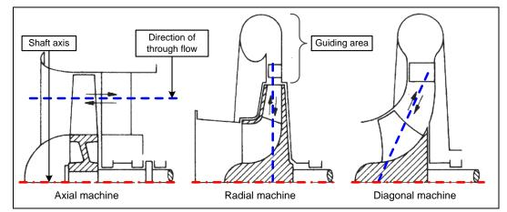
Figure 4.3: Direction of through flow for axial, radial and diagonal machines
