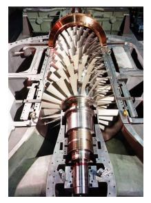
Figure 1.4: Axial compressor
