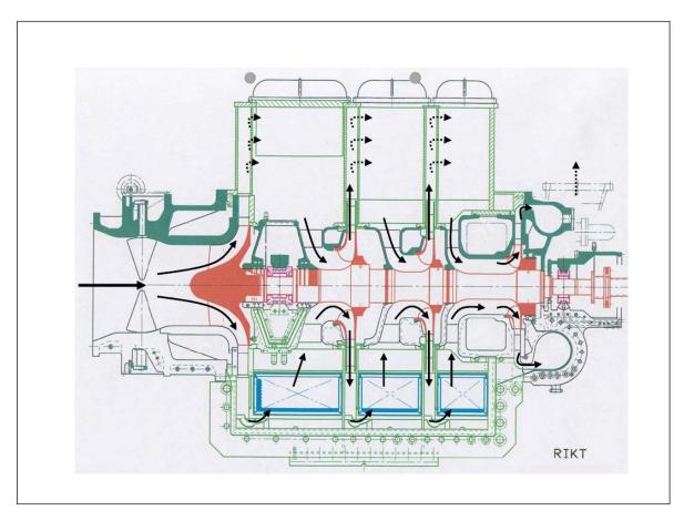
Figure 4.8: Schematic structure and flow profile of RIKT
