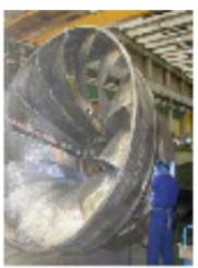
Fig 1.8: work on a Francis impeller
