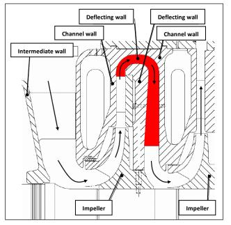
Figure 4.26: Channel, intermediate and deflecting wall
