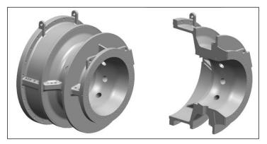
Figure 4.19: Inlet casing without prerotation
