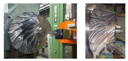
Figure 4.11: Milling impeller 1<sup>st</sup> stage
