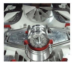
Figure 4.16: Combined journal-thrust bearing and bearing housing
