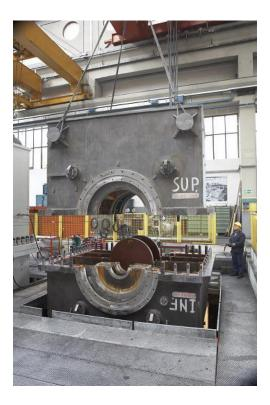
Figure 2.5: preparation for the hydraulic pressure test
