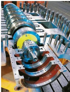
Figure 4.6: Centrifugal compressor with horizontal split design
