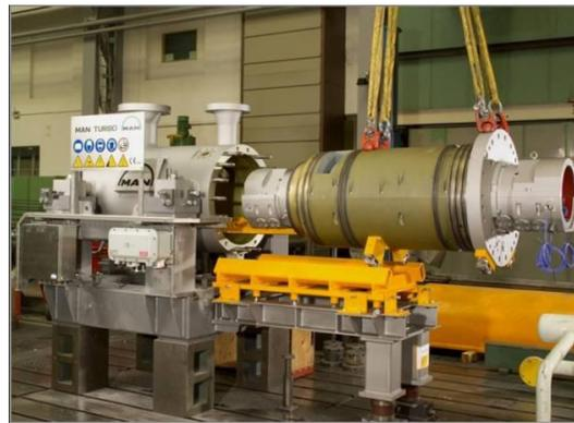
Figure 4.7: Centrifugal compressor with barrel design
