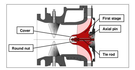
Figure 4.12: Sectional view 1<sup>st</sup> stage
