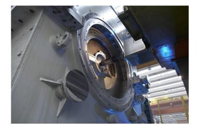
Figure 2.4: boring machine PAMA 200 working in the bearing zone of a RIKT
