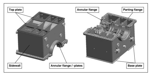
Figure 4.22: Main parts of the outer casing
