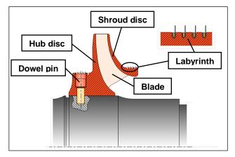
Figure 4.14: Sectional view labyrinth strips
