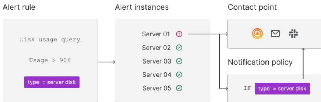
Figure 4.6: Grafana Alerting diagram. Source: [15]
