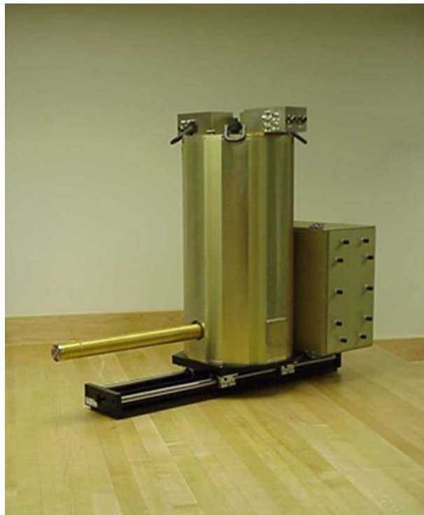
Figure 1.6: One of the first developed STJ detectors
