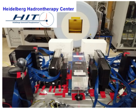
Figure 3.1: Four i-TED modules placed in front of each other with the target in the middle, allowing for use of both Compton and PET imaging. Image during a study under clinical conditions at the Heidelberg Hadrontherapy Center.
