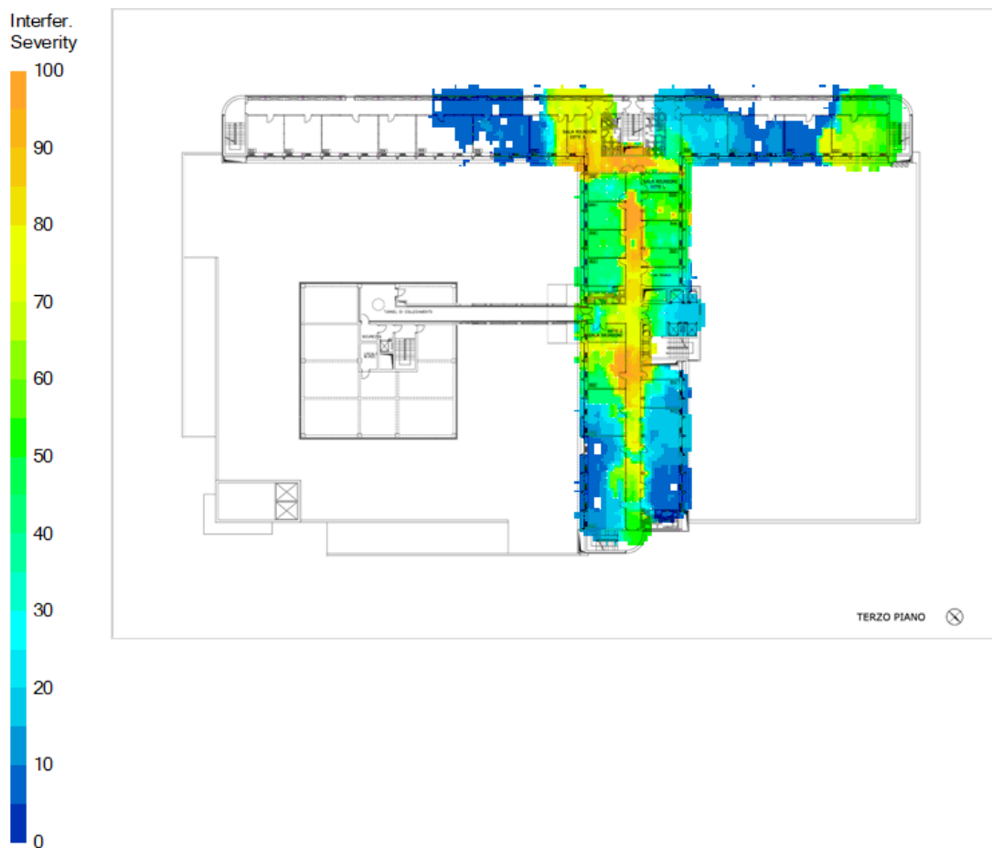
Figure 7.27: Interference level of the new infrastructure on 2.4 GHz band
