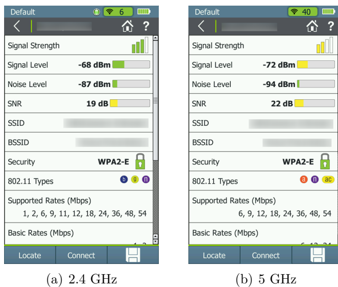
Figure 7.15: Signal level received by the Aircheck G2 on room DITE 2
