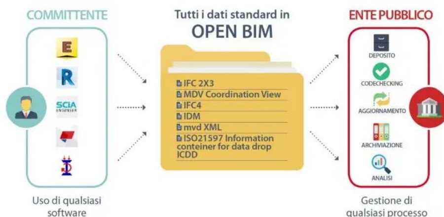
Figura 53 - Structural E-Permit e Open BIM
