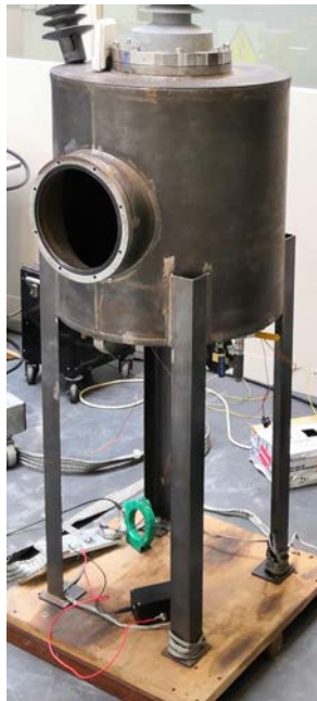
Figure 3.2: Pressure vessel in the HV laboratory.
