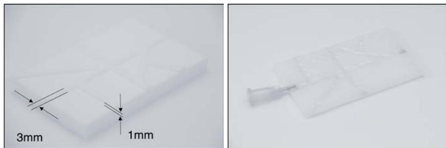
(a) Mold used for ecoflex casting
