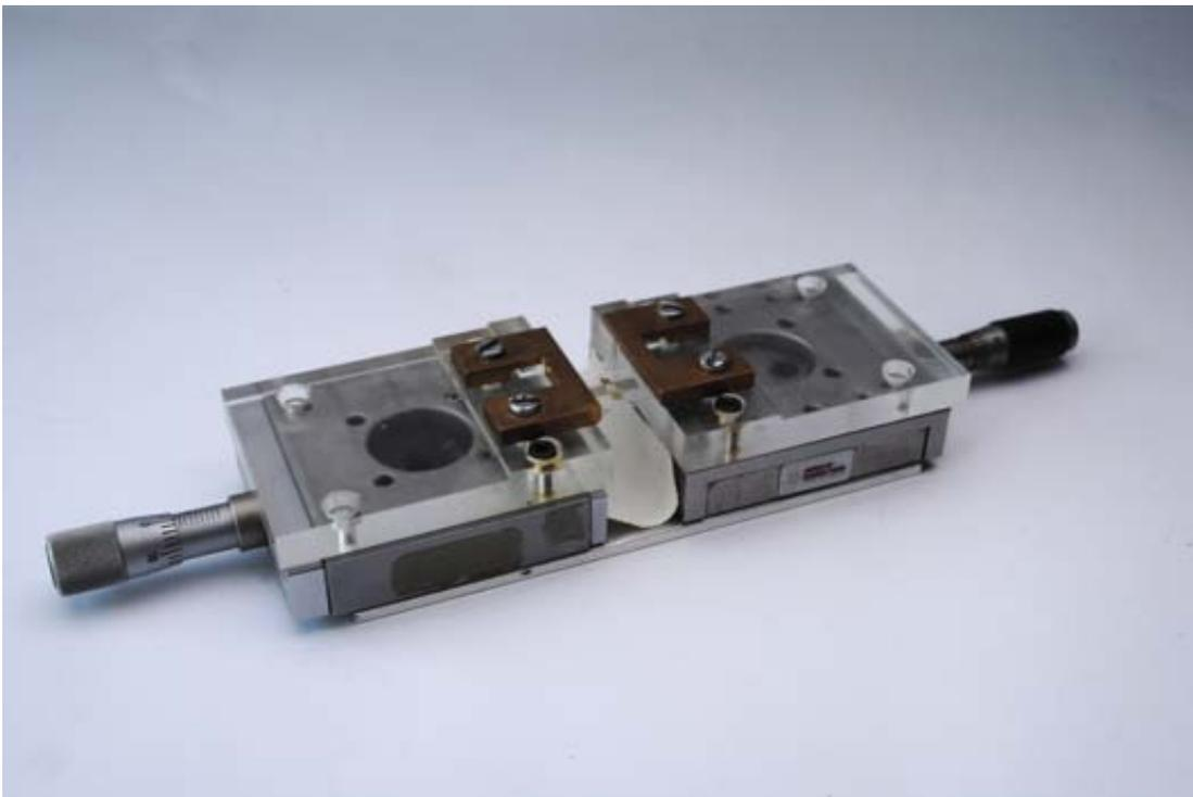
Figure D.1: Stretching setup used for testing.
