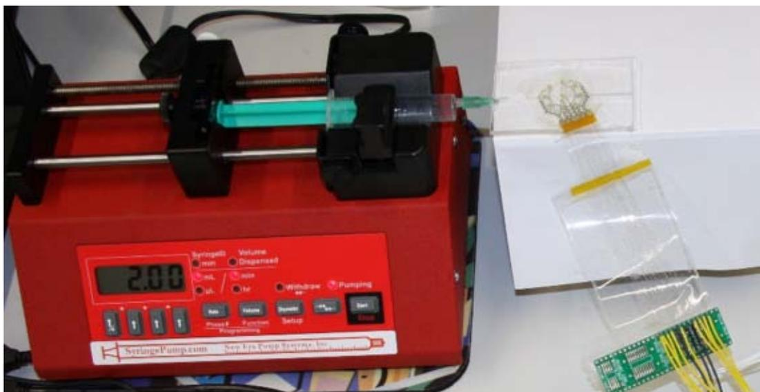
Figure D.2: Setup used for liquid flow testing.
