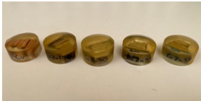
Figure 3.4 Samples of copper and CuZn alloys mounted in resin.
