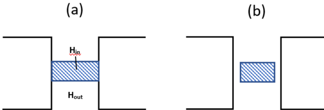
Figure 5.15 Example of (a) closed and (b) open magnetic circuit.
