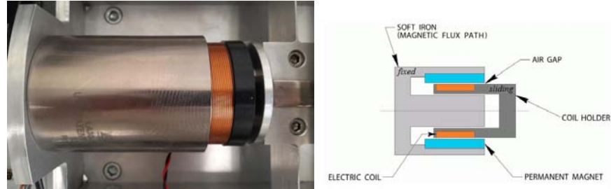
Figure 3.7: Voice Coil Actuator: Photo and Scheme [23]
