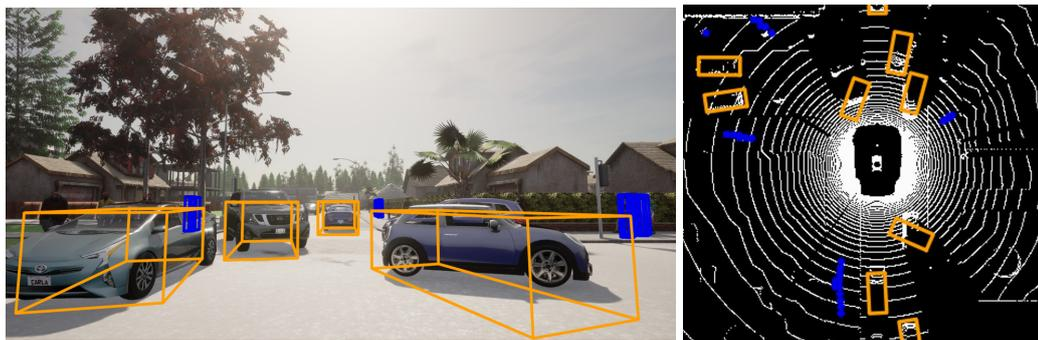
Figure 5.4: Front view (left) and BEV (right) of predicted bounding boxes of camera-only model.
