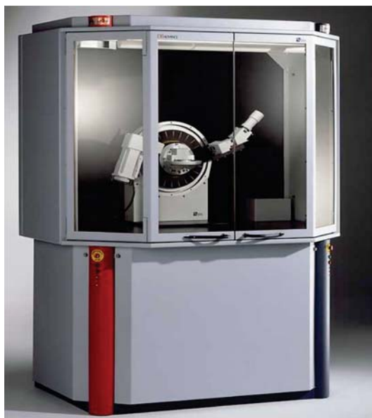
Fig. 4.1 BRUKER®D8 ADVANCE instrument for powder diffraction.
