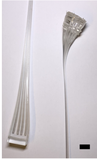
(a) Initial drop and residual preform after the thermal drawing, with a ruler for scale.
