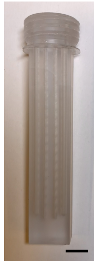
(b) The second PC-W preform, with enlarged side holes. Scalebar = 1 cm.
