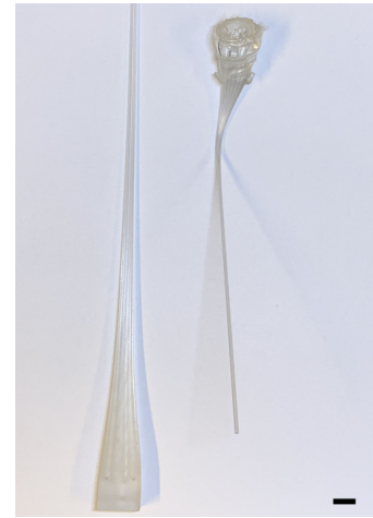
(c) Initial drop and residual preform after the thermal drawing. Scalebar = 1 cm.
