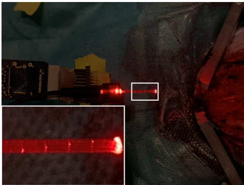
(b) Top view of the first implant, before the contact with the spinal cord. The four scattering points are magnified in the inset.
