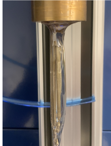
(b) Residual of the preform after drawing. The distorted shape shows that the draw temperature was too high for the polycarbonate.
