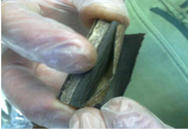
Figure 1.II.2: commercial Ni-MH battery. The anode is plated on a Ni foil and rolled with a separator impregnated of basic solution and two Ni hydroxide layers,
