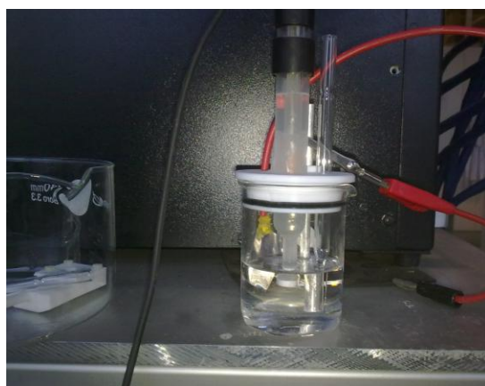
Figure 2.IV.3: The Three electrodes setup assembled and preliminary tested at the TU Delft
