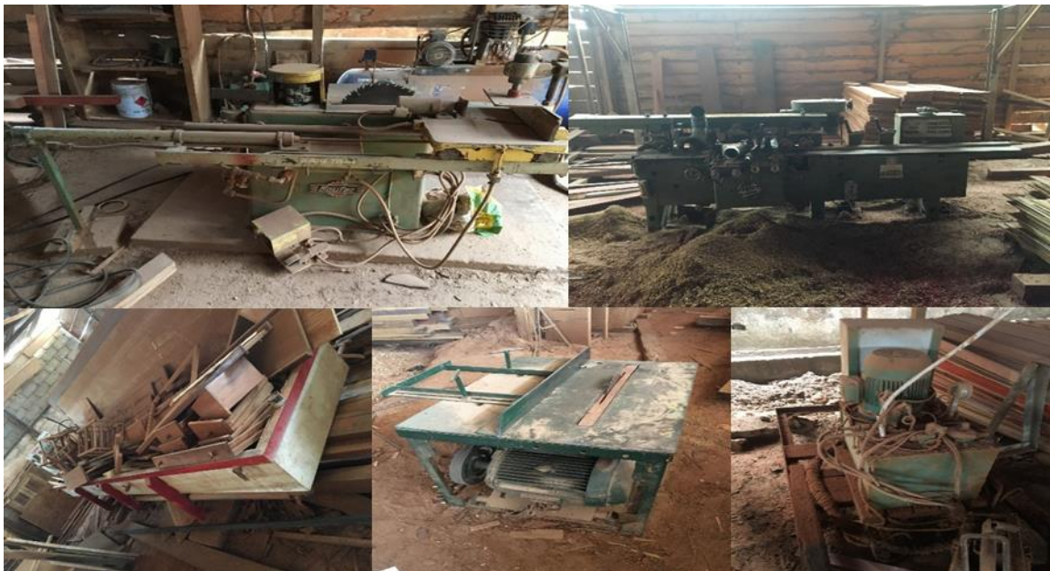
Annex 16: Some GLT manufacturing machines from top-left to bottom-right; splinting machine, four-side moulder, vacuum wood drying machine, circular saw table machine and hydraulic press.
