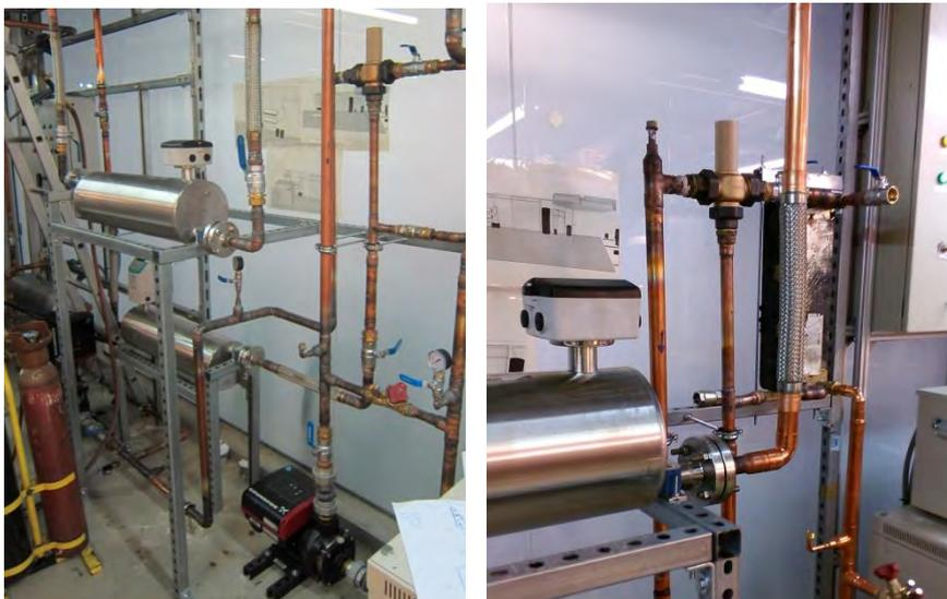
**Figure 36: From the right, coriolis installation in detached supports and under head, in the figure could be seen also the flexible sections; detail of one flexible section.**
