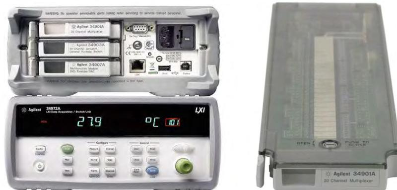
**Figure 39: In the right the front and the back of a data logger used in the installation, in the right one of the three slots present in every data logger**
