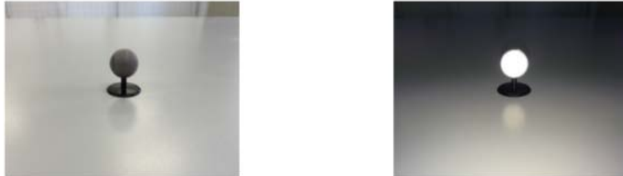
Figure 2.3: the left image shows a marker exposed to the ambient light. To the right we can see a marker exposed to a digital camera flash
