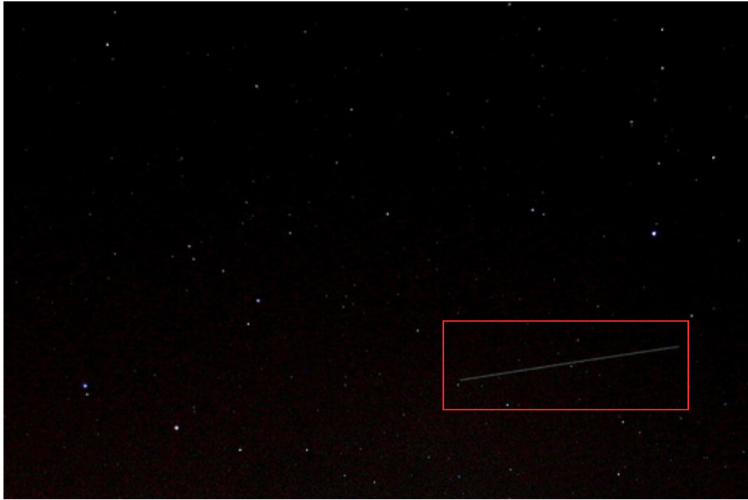
Figure 4.1: A satellite streak amongst a field of stars acquired in staring mode. Credits: John McGraw, “Angles and Range: Initial Orbital Determination with the Air Force Space Surveillance Telescope (AFSST)”
