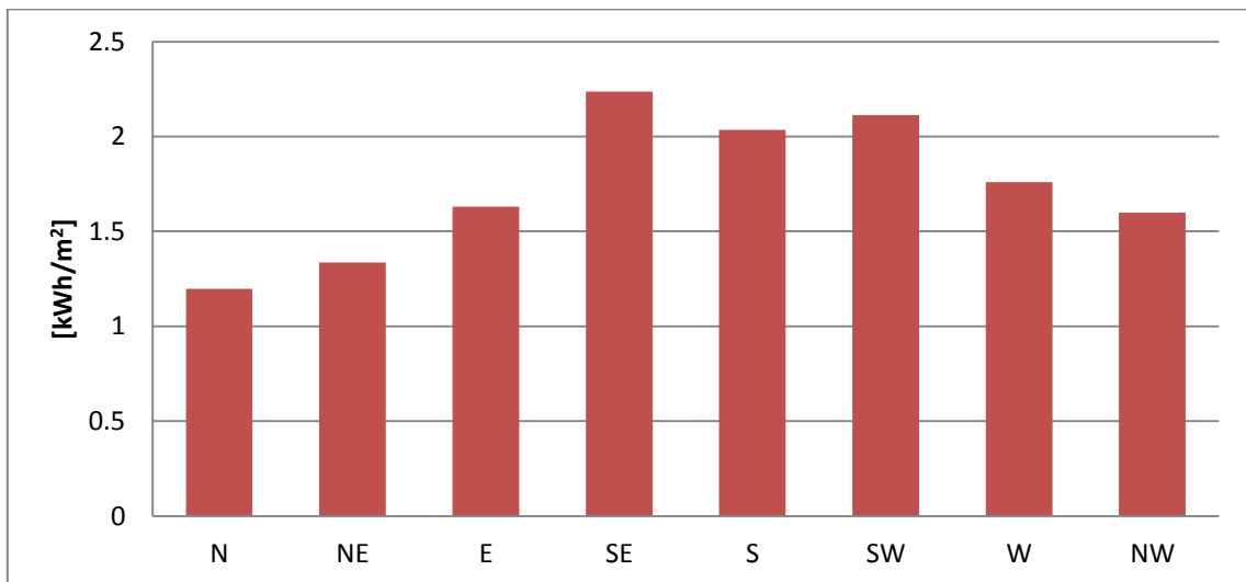
Figure 111 – Energy consumption for the tested orientations.
