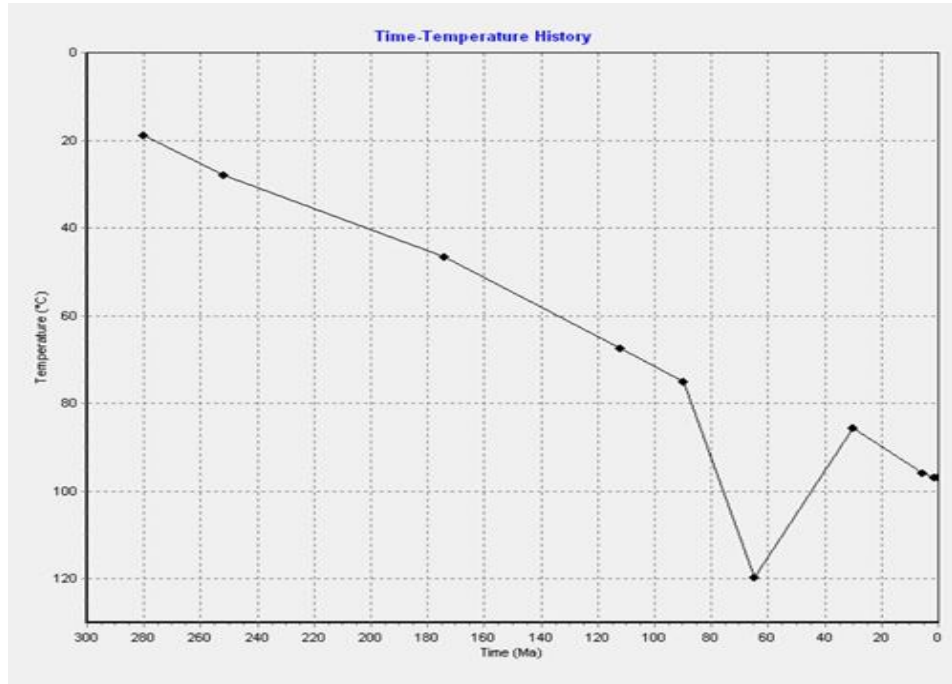
Fig. A37. Thermal history of the well BR_LT 3014 with temperature reduced of the 5%. Ketcham et al., 2007a and Laslett et al., 1987 equations have been used to determine AFT ages and Farley, 2000 and Flowers et al., 2009 equations have been used to determine AHe ages.
