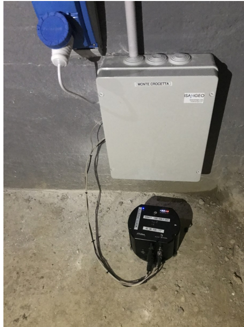
Figure 86: Seismometer deployed on the rigid concrete floor
