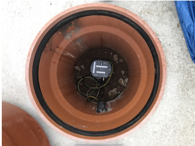
Figure 81: Triton Seismometer with corner frequency of 1 Hz, placed after removing 1 meter of top soil
