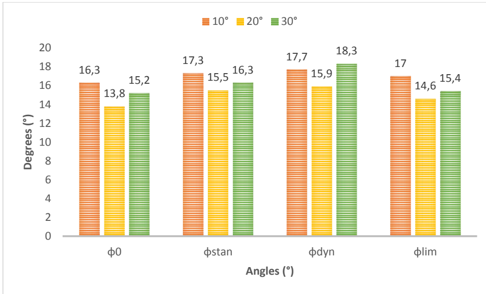
Figure 6.28. IP tests at different temperatures, GNT-GMB interface.
