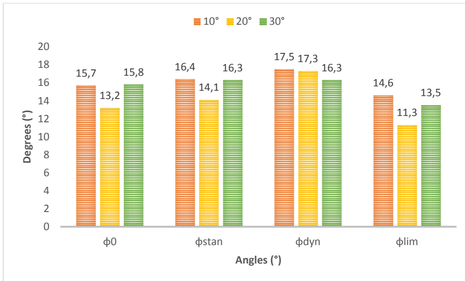
Figure 6.27 IP tests at different temperatures, GTX-GMB interface.
