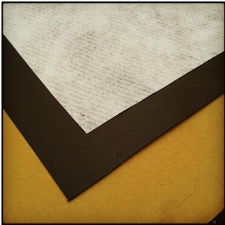
Figure 5.10.a. Geosynthetics and interfaces tested: 1) GTX-smooth GMB HDPE; 2) GNT-smooth GMB
