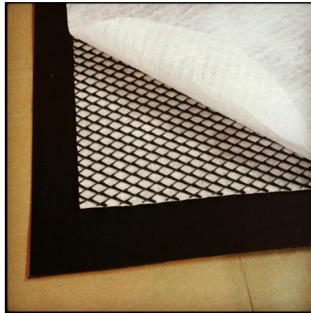
Figure 5.10.b. Geosynthetics and interfaces tested: GMB HDPE; 3) GCD- smooth GMB HDPE.
