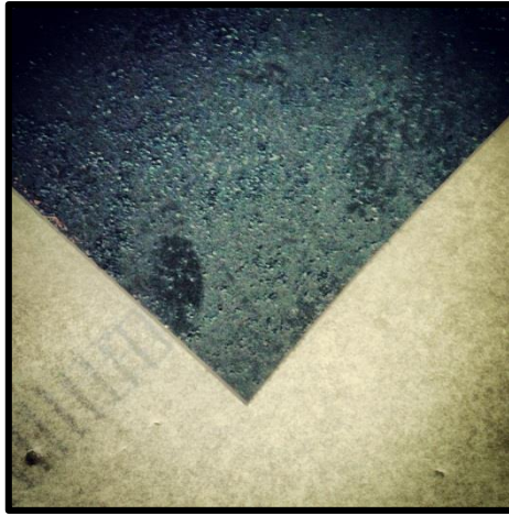
Figure 5.11. Geosynthetics tested: textured GMB HDPE.
