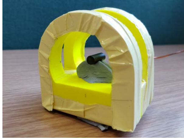
Figure 3.13: The apparent permeability \mu_a was calculated by measuring the B field on the surface of the core placed inside the known H field generated by the Helmholtz coil.
