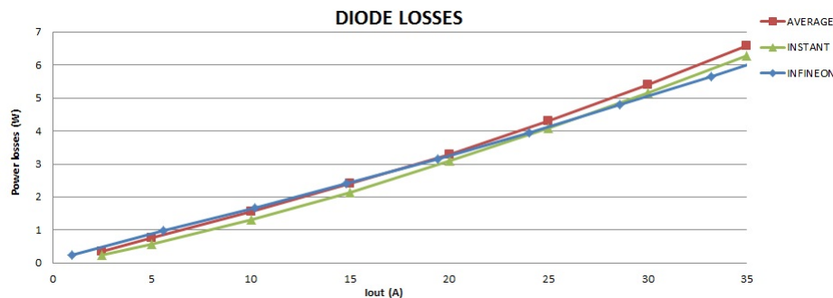
Figure 3.5: Diode's power losses function of the current
