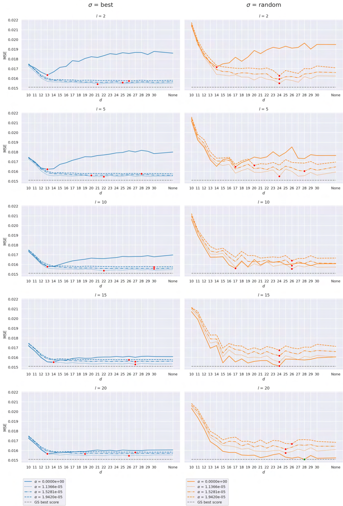
Figure B.4: Generalisation MSE estimates of the regression trees explored when combining different pruning techniques and splitting approaches of the predictor space. Red dots denote the minimum of each curve and, the green dot identifies the score of the best-performing regression tree.
