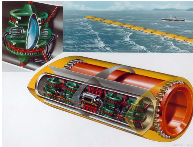
Figure 9 - The Duck version of 1979 equipped with gyroscopes (courtesy of University of Edinburgh)
