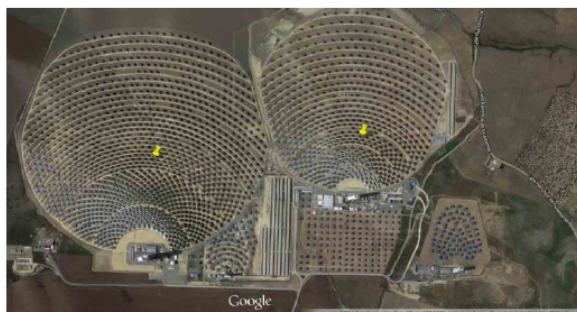
Figure 1.17: Tower at the vertex of the heliostat field (PS 10 and PS20 plant, Spain) [20]
