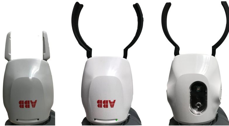
Figure 10.10: Standard gripper (on the left) compared to the special ones used (on the right).
