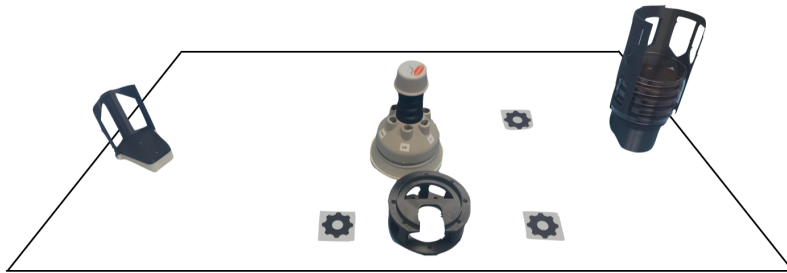
Figure 10.12: Scheme of a fixed workstation with features to retrieve the task frame.
