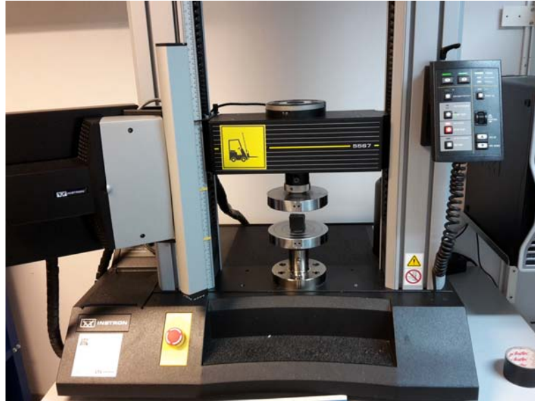
FIGURE 4.4: Specimen undergoing a compression test with an Instron 5567
