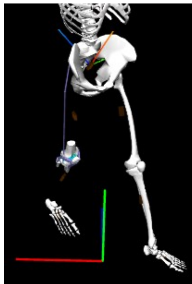
Fig. 4.8 IMU IK shows that the forward direction is not the same as the one of the MoCap system (along x positive axis). The model is rotated of an angle about the y-axis of the Opensim frame.
