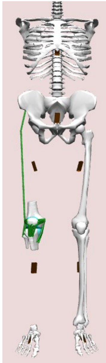
Fig. 4.6 Output of the IMU placer tool , model updated with IMUs with the correct orientation on each body segment. To avoid confusion all muscles have been hidden.
