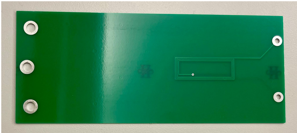
Figure 3.4: PCB coil used to perform the voltage measurements
