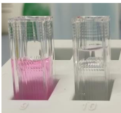
Figure 3.10 Cuvettes containing RhB solution without catalyst (left) and MM4-RhB solution at the end of the experiment (right).
