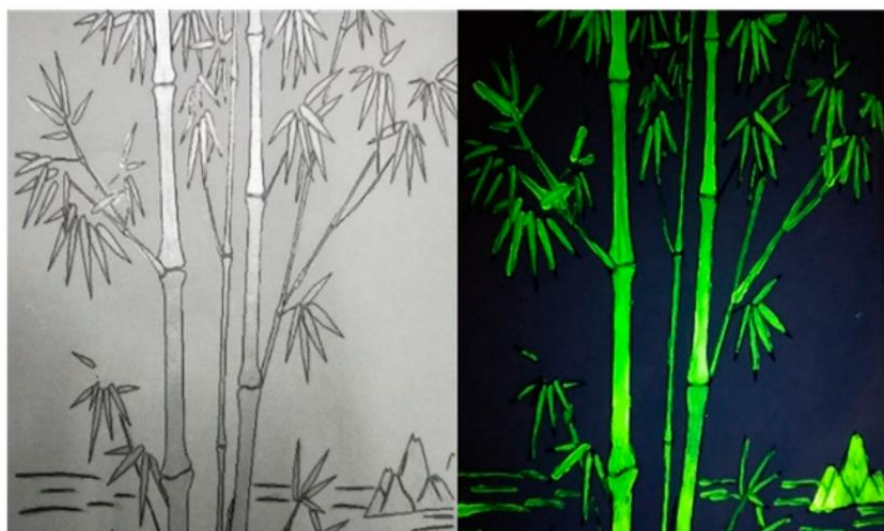
Figure 1.20 A picture painted by the \text{Cu}_4\text{I}_6(\text{pr-ted})_2/\text{PVP} ink under natural light (left) and 365 nm ultraviolet light (right) 16 .
