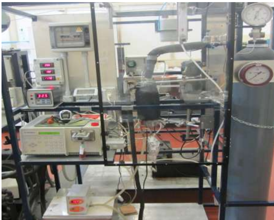
Figure 2.4 Picture of the pilot plant used to perform the precipitation of antioxidant from cherries extracted solution.
