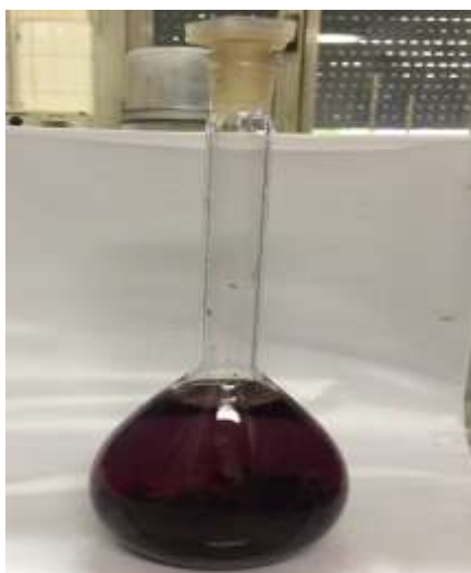
Figure 2.2 Extracted sample before the centrifugation.
