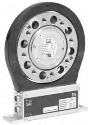
Figure 6.4: Torque meter: HBM T40 ; Analog voltage output ; Sensitivity: 10 mV/Nm ; Bandwidth: 6 KHz ; Accuracy: \pm 1 Nm. Source: [29]
