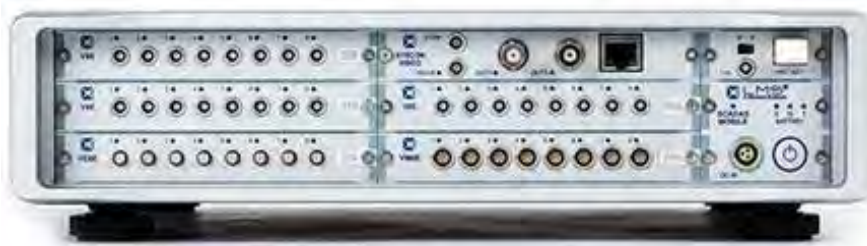
Figure 6.2: Acquisition system: LMS SCADAS Mobile 05; 24 bit ADC sampling at 204.8 KHz; 820 MHz frequency clock, yielding 1.2 ns time resolution; 1 MHz maximum input pulse rate in digital mode. Source: [29]
