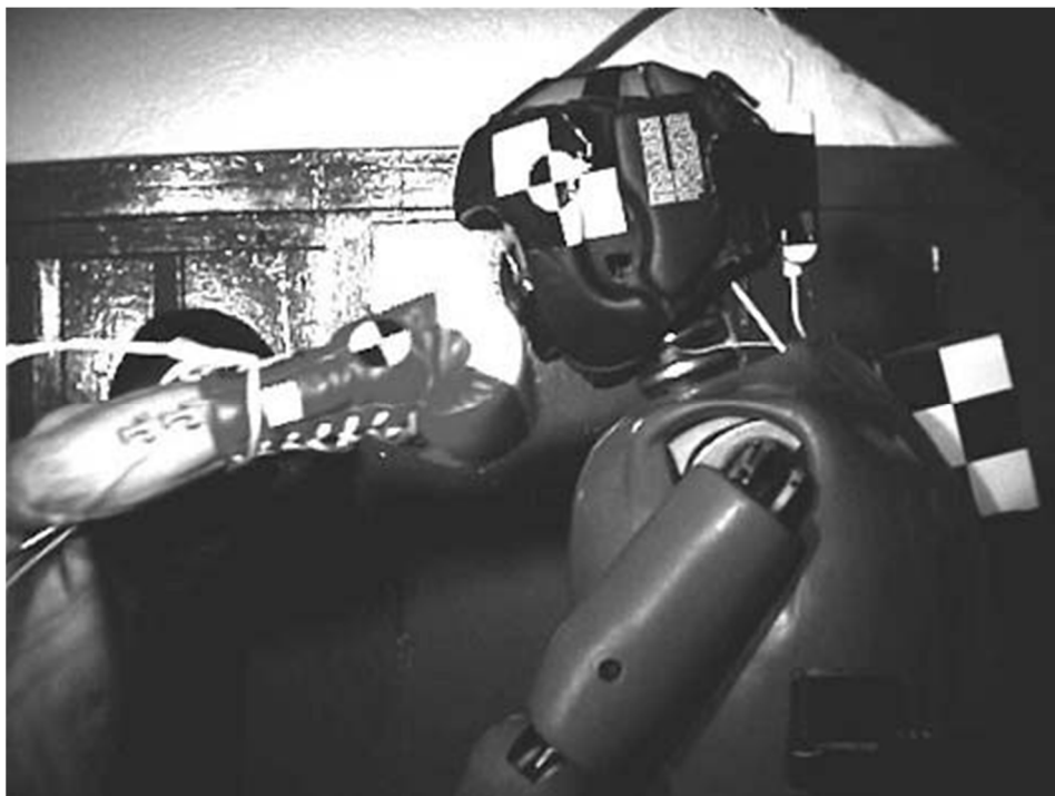
Figure 3. Olympic boxer throwing straight right punch to jaw region of instrumented Hybrid III dummy [19]
