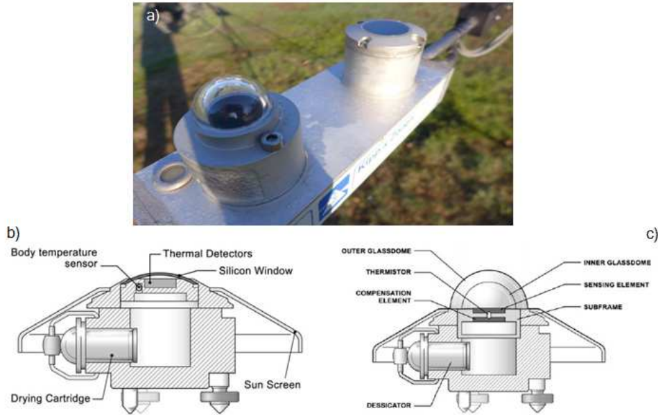
Figure 6: a) Kipp and Zonen net radiometer model CNR1 [20], b) Kipp and Zonen CG4 pyrgeometer [19] and c) Kipp and Zonen CM11 pyranometer schematic construction [18]
