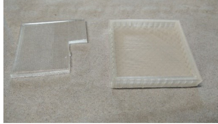
Figure 22: PLA 3D printed micropattern piece (right side), and the demolded PDMS piece after curing (left side)
