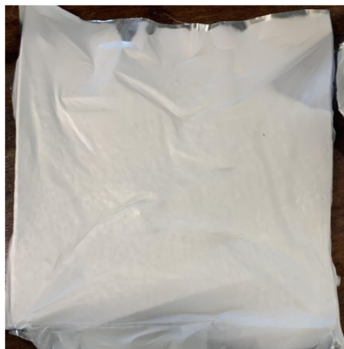
Figure 28: an electrospun mat obtained with the described standard procedure
