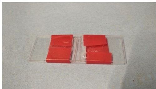
Figure 21: the structure for a sample before injecting the cross-linking solution
